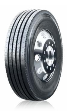
The S606 is Sailun's premium steer tire, featuring extra wide shoulders with built in sipes for excellent stability and traction under all weather conditions. An extra deep 22/32" tread depth ensures the S606 delivers exceptional mileage, while an interlocking symmetrical tread block design promotes even wear and a square footprint.
