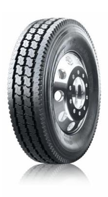
The S768 EFT is a premium closed shoulder drive tire, designed with a wide shoulder featuring tapered lateral edges for enhanced lateral stability. The S768 also features stone ejector buttons that reduce stone retention, and an extra-deep 26/32" tread depth for enhanced tread life.
