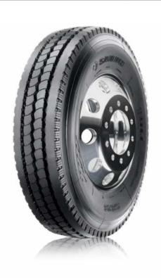
The S828 is good for highway, common road, long-distance transport, as well as all wheel axles. Three longitudinal grooves and horizontal shallow sipes provide the tyres with both good maneuverability and drivability. High-intensity crown and carcass design improves tire resistance to bursting and ensure driving safely.
