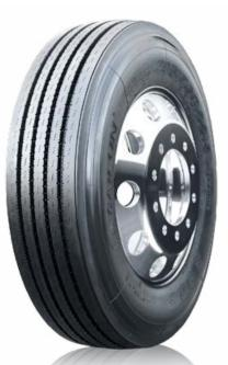
The S605 is Sailun's premium long-haul steer tire, featuring a decoupling groove and five wide ribs for a stable ride at all speeds. Stone ejectors minimize tire damage, while extra-wide grooves and S-sipes effectively disperse water for excellent hydroplaning resistance.
