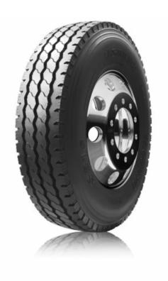
The S816's unequal pitch of tread patterns is designed to reduce the rolling noise of the tyre. The reinforced carcass and reinforced tire bead make the service life of a tyre longer. Its closed shoulder is used both to guarantee its good stability and reduce the abnormal wear of its shoulder.
