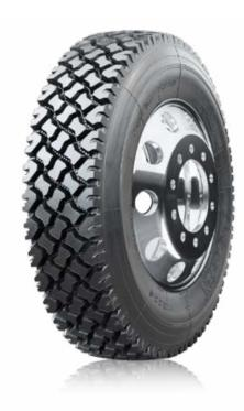
The S758 is designed for severe off-road applications. With an extra-deep 32/32" tread depth and a rubber compound engineered to resist the most demanding environments, the S758 is ideal for construction, logging, and off-road environments. Stone ejectors resist the damages caused by stone retention, and an open shoulder with tapered sidewalls aids lateral stability.
